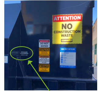
Compactor Hatch With Safety Interlock
